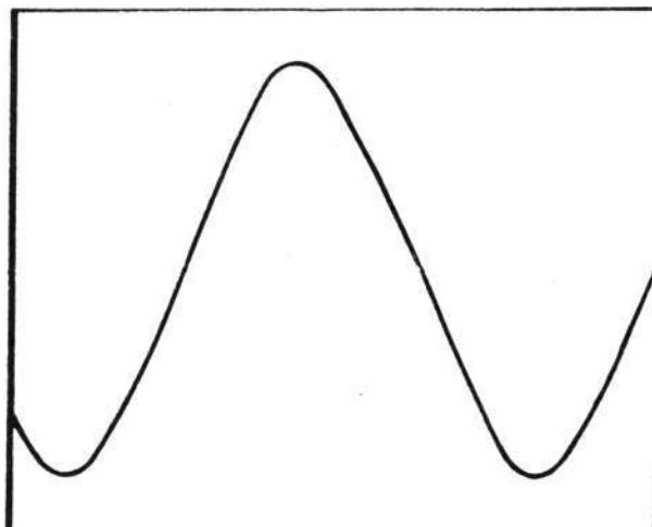
14. Place the probe tip on TP9. Check that the display shows the same waveform as in step 13.
