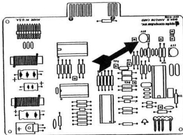
17. After you have made the adjustments, turn the Apple ][ off. Then disconnect the customer's drive, apply Glyptol to the potentiometers, and re-assemble the drive.
